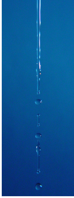
Figure 2: The capillary-driven instability of a water thread falling under the influence of gravity. The initial jet diameter is approximately 3 mm.
