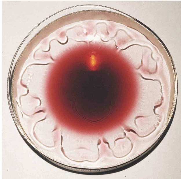
Figure 1: The tears of wine. Fluid is drawn from the bulk up the thin film adjoining the walls of the glass by Marangoni stresses induced by evaporation of alcohol from the free surface.
